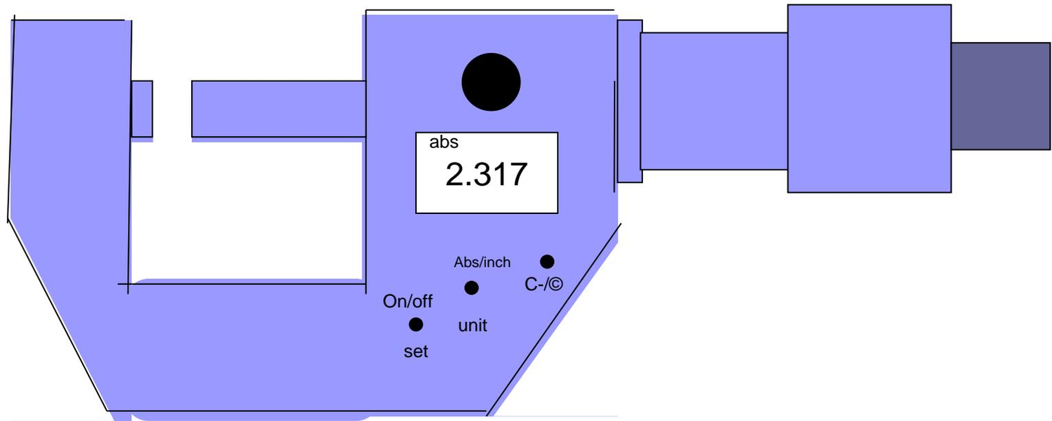
Using **only the ratchet** close the caliper.
