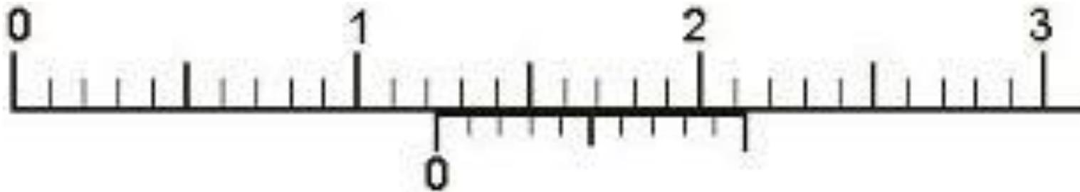
The level of precision depends on the ***difference*** between the size of the smallest division on the **main scale** and the size of the smallest division on the **Vernier scale**.
