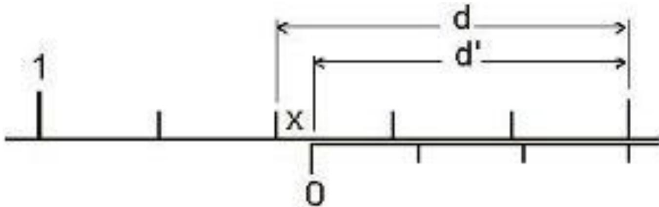
The vernier part of the reading is really a subtraction:
