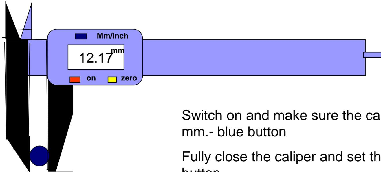
Switch on and make sure the callipers are set in mm.- blue button
